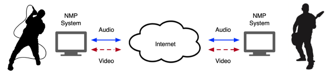
Fig. 5. A diagram of the dataflow exchanged during a NMP between two geographically displaced musicians.
