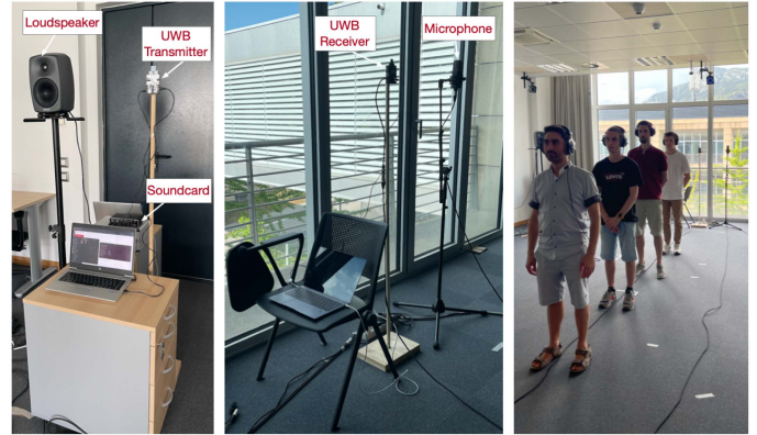
Fig. 3. Transmitter (left) and receiver (middle) apparatus; NLOS setup (right).
