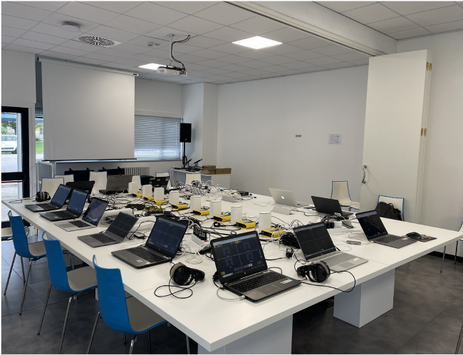
Fig. 3. Picture of the simulation environment of the 5G architecture, showing the base station, the nine CPEs, the eight NMP devices, the eight headphones, the soundcard, the 13 laptops, and the smartphone.
