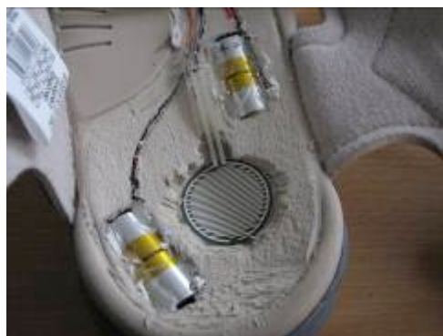
Figure 3. A picture of one pressure sensor and two actuators embedded in the shoes.
