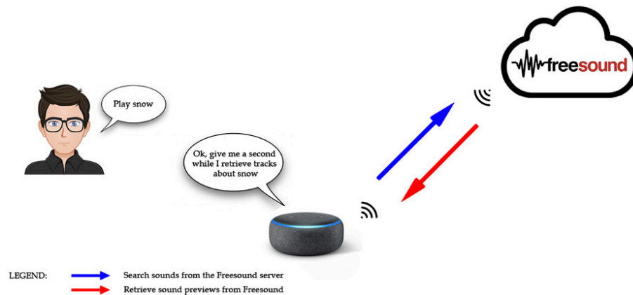
Figure 1: Schematic representation of the implemented Internet of Audio Things ecosystem.
