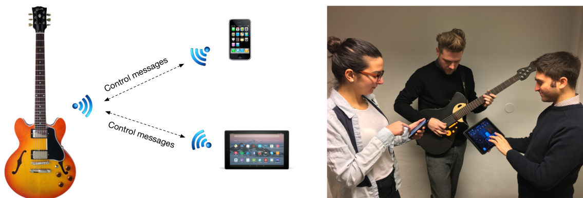
Figure 1. A schematic representation (left) and a picture in a real setting (right) of a jam between three musicians involving the Sensus smart guitar and dedicated apps running on an iPad Air 2 and an iPhone 6s.
