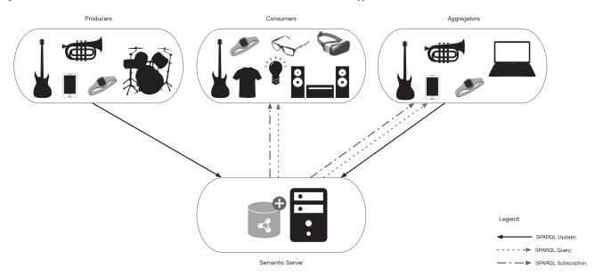
Fig. 2. Schematic representation of an example of ecosystem based on the proposed semantic IoMusT architecture. Different types of Musical Things play different roles of producer, consumer, or aggregator
