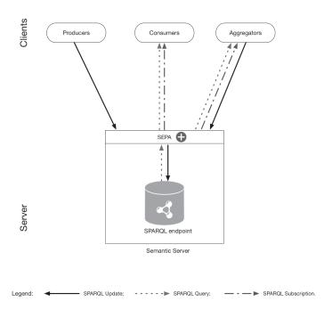
Fig. 1. The semantic IoMusT architecture, based on a client/server architecture of a SEPA application
