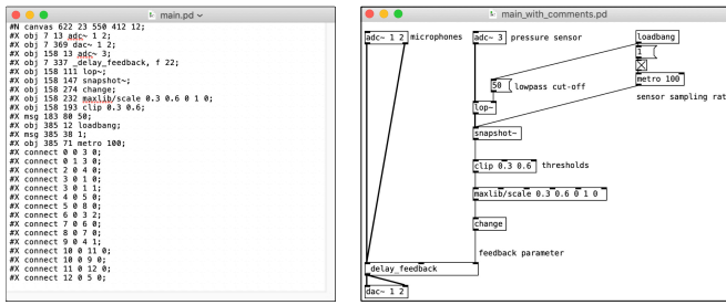
Fig. 3. The generated Pure Data code and its graphical representation as a patch (comments added afterwards for clarity's sake).
