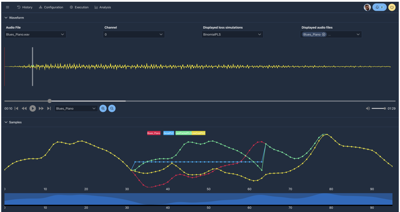
Fig. 6. The waveform can be zoomed in to the sample level. Additionally, there is a convenient view below the main waveform that is centered on the lost packet. Both views can display multiple waveforms at a time, allowing the comparison of different PLC algorithms.
