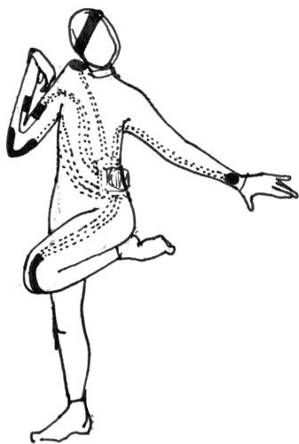
Figure 1: Sketch of a performance, using integrated textile sensors on joints to create sound from body movement.
