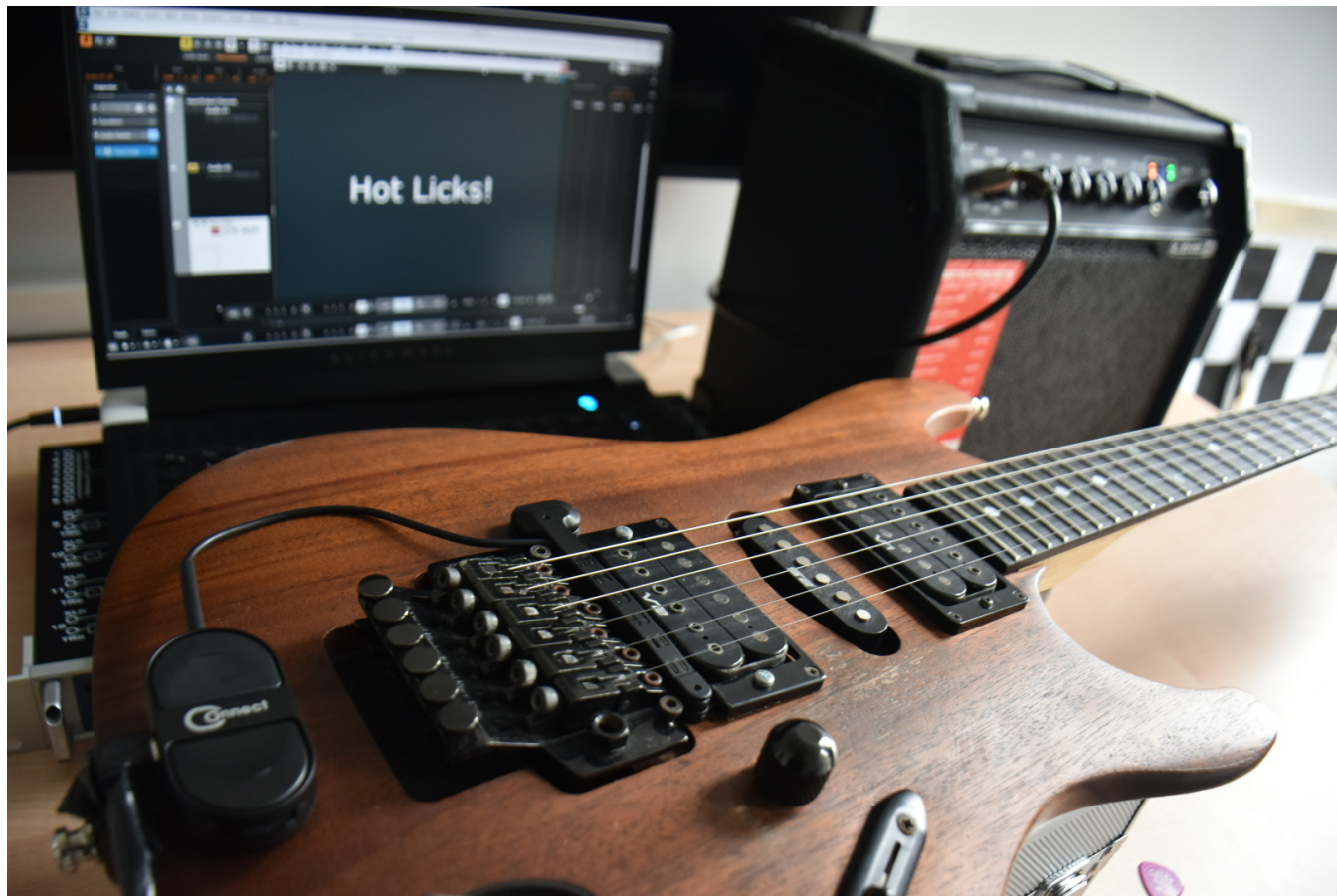
Figure 1: The smart electric guitar outfitted with the MIDI Tracker.
